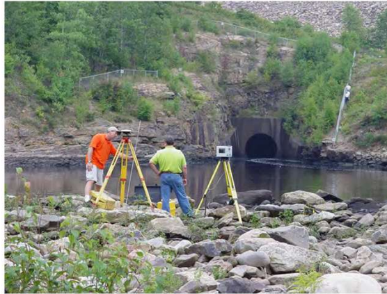
Figure 31: Optech Iris Unit positioned in center of river bed at the Francis E. Walter Dam site located in Whitehaven, Pennsylvania.
