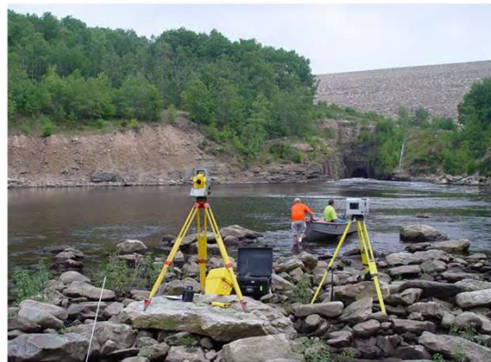
Figure 32: Reflecterless Total Station was utilized to georeference scanner data to project control network.
