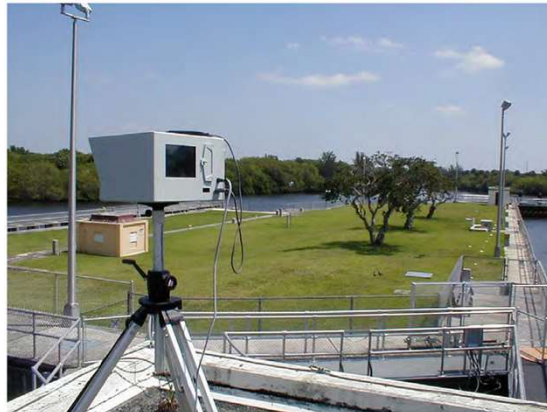
Figure 19: Optech ILRIS 3D laser scanner--detailed mapping of structures and facilities at St. Lucie Lock and Dam, Jacksonville District.
