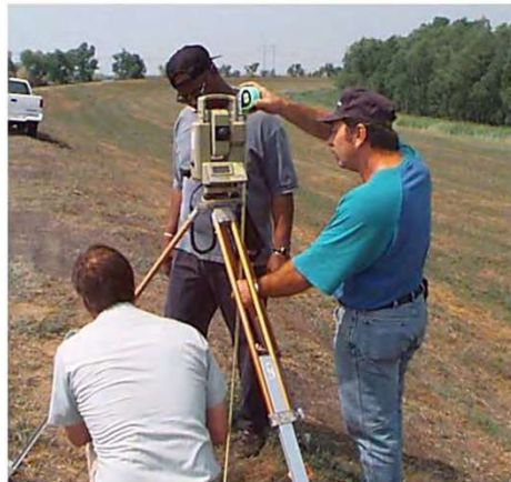
Figure 1: Wild TC-1010 Total Station with TDS-HP48GX Data Collector 1998 Levee Survey at Bayou Segnette.
