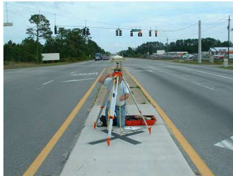
Figure 11: Static or Fast-Static survey techniques. Rover is set on a tripod accurately centered over a control point or feature such as a photo target. 5 minutes to 2 hours of static data may be collected whereas an RTK solution may have only a few seconds using a hand-held antenna pole.
